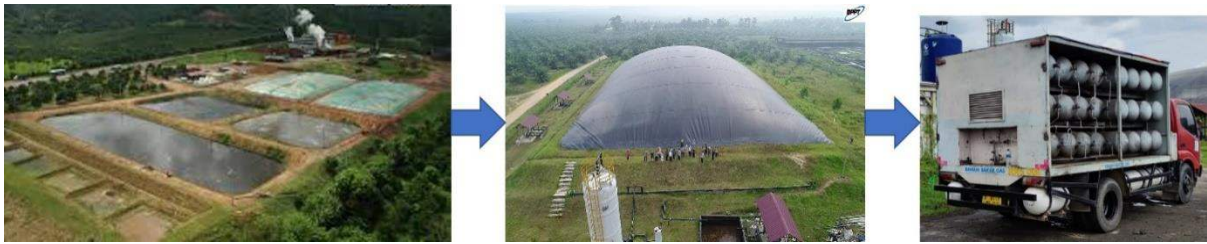
Figure 29 Schematic Illustration of POME Conversion to Biomethane for Fuel of Palm Oil Plantation Trucks 29
